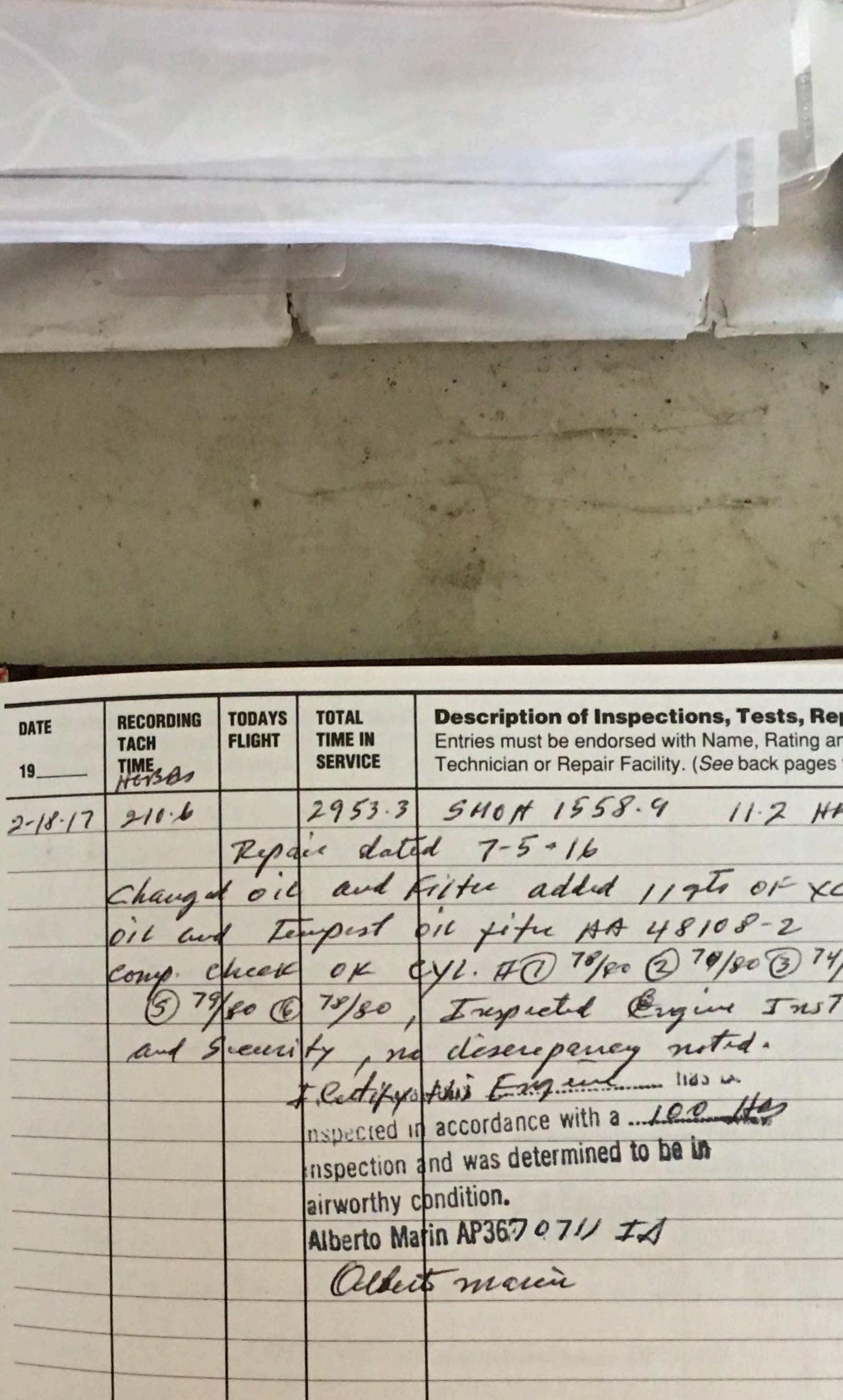
**Description of Inspections, Tests, Repairs and Alterations** Entries must be endorsed with Name, Rating and Certificate Number of Technician or Repair Facility. (See back pages for other specific entries.) 11.7 HPS since last Filte added 11gts of XC 20-50 philips EVI. ATO 78/00 @ 79/80 374/80 (4) 74/80 Inspected Ergine Installation, condition noted . © 1991 ASA
